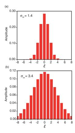
FIG. 5. (Color online) Calculated OAM mode spectrum for the two measured distribution widths of (a)  $\sigma_m = 1.4$  and (b)  $\sigma_m = 3.4$ . The normalized amplitude is plotted as a function of OAM mode number  $\ell$ .
