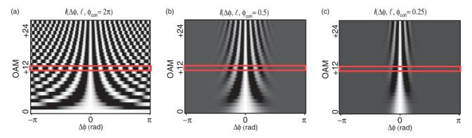
FIG. 2. (Color online) Simulation results for angular interference patterns for OAM mode projections from  $\ell=0$  to  $\ell=24$  for three values of coherence angle (a)  $\phi_{\rm coh}\approx 2\pi$  rad, (b)  $\phi_{\rm coh}=0.5$  rad, and (c)  $\phi_{\rm coh}=0.25$  rad. The red rectangular boxes indicate the value of  $\ell$  used in our experiment. The z axis shows normalized intensity from 0 to 1, indicated by grayscale values.
