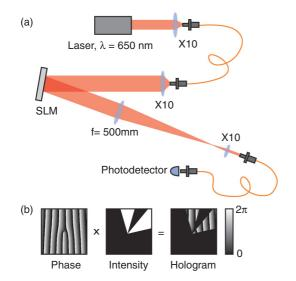
FIG. 3. (Color online) (a) Schematic of the experimental setup. (b) Example of a phase hologram impressed on the SLM.
