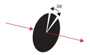
FIG. 1. (Color online) Partially coherent field propagating through double angular slits with an angular separation of  $\Delta\phi$ .
